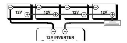
Series connecting increases the voltage in a system, while capacity of the battery bank remains the same. Here is an example of series connecting four batteries together to create a 48volt system, and a 24volt system. Then paralleling the 24 and 48volt banks with another 24 and 48volt bank to increase capacity.
